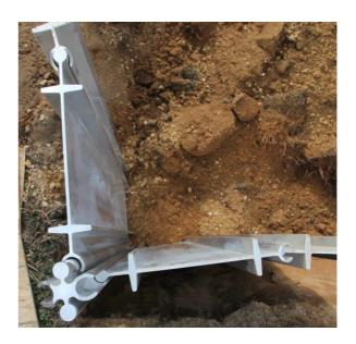
The panels are made of fully extruded 6061 T6 aluminum, and weigh 10lbs. per foot (for example: 5' = 50lb and 8' = 80lb). Panels come in 5' and 8' sections (or any custom length in between) with an effective 16 inch width. Knuckles come in 8 foot sections. Panels stack in a compact configuration for easy transport.
